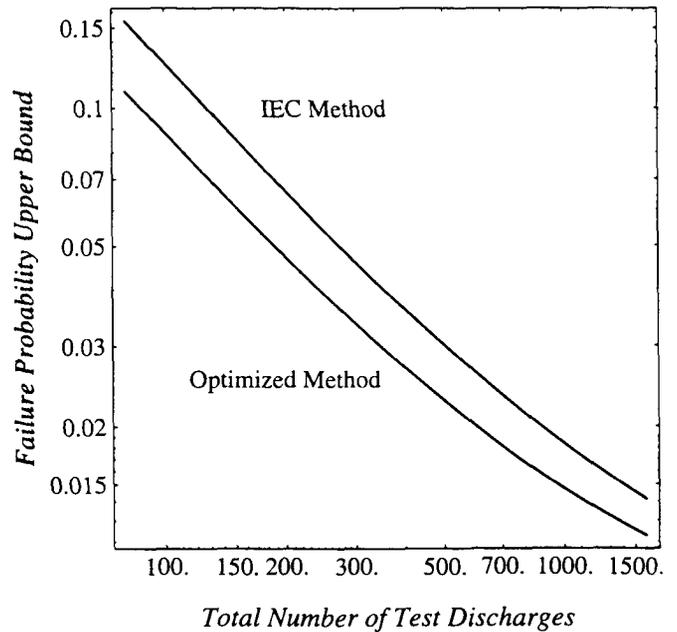
**Figure 4.** Failure Probability Upper Bounds Versus ESD Tests (No Measured Failures)
