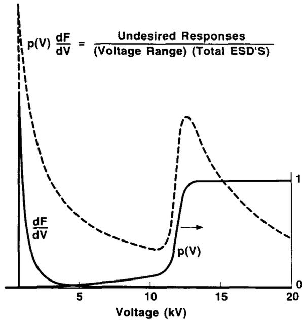
Figure 1. Typical  $p(V)$ ,  $dF/dV$  and Failure Distribution Curves
