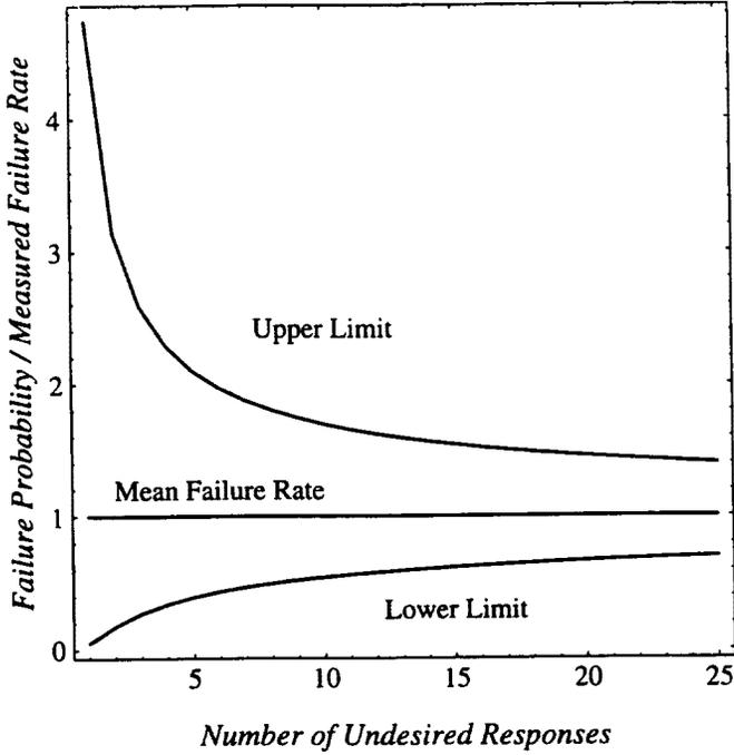
Figure 2. Ratios of Failure Probability Limits to Measured Failure Rates
