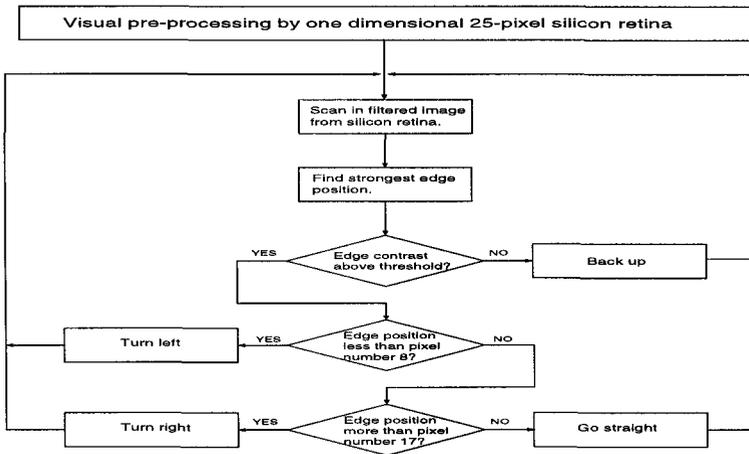
**Fig. 2.** The simple tracking controller structure implemented on Koala, which gives a good performance in conjunction with the “cheap” but sophisticated analog VLSI sensory processor.
