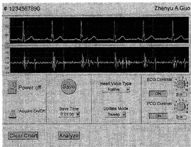
Figure 2. Main PCG panel. Live ECG and PCG signals are displayed. Two knobs are used to control the ECG and PCG gains. ECG and PCG signals can be saved by clicking the Save button. The valve types can also be selected.
