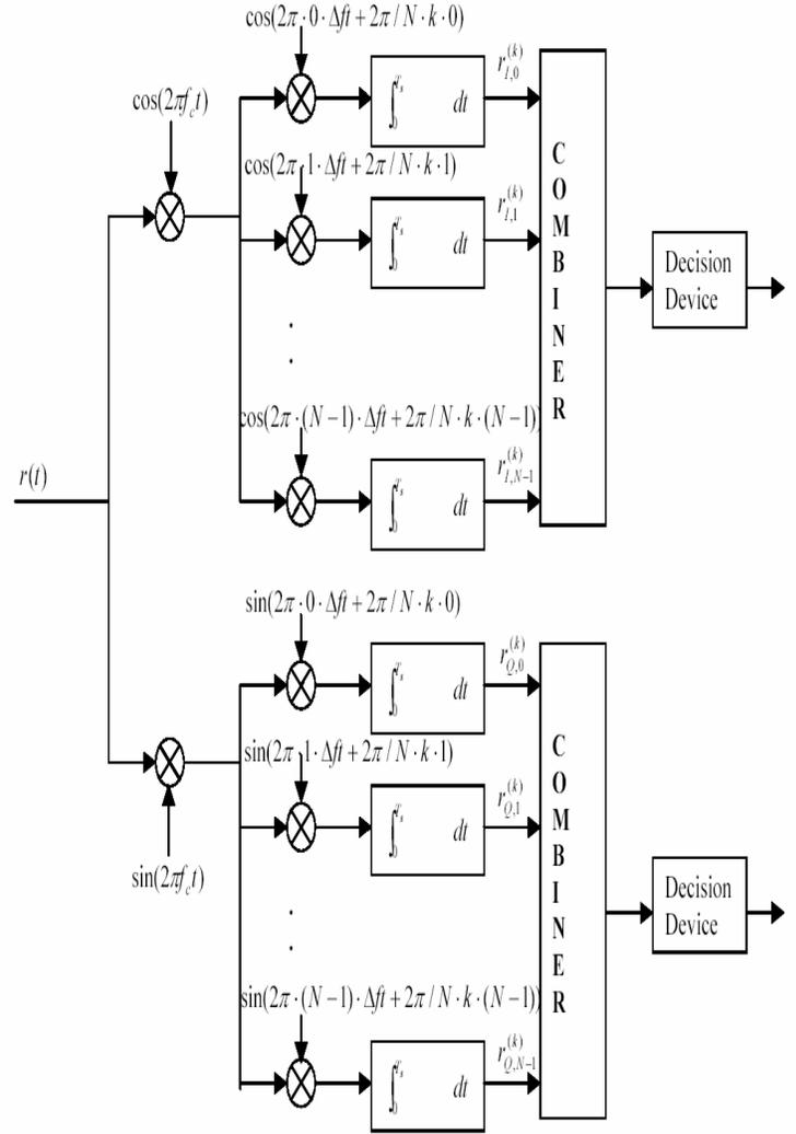
Figure 2. Receiver for CI/OFDM with QAM
