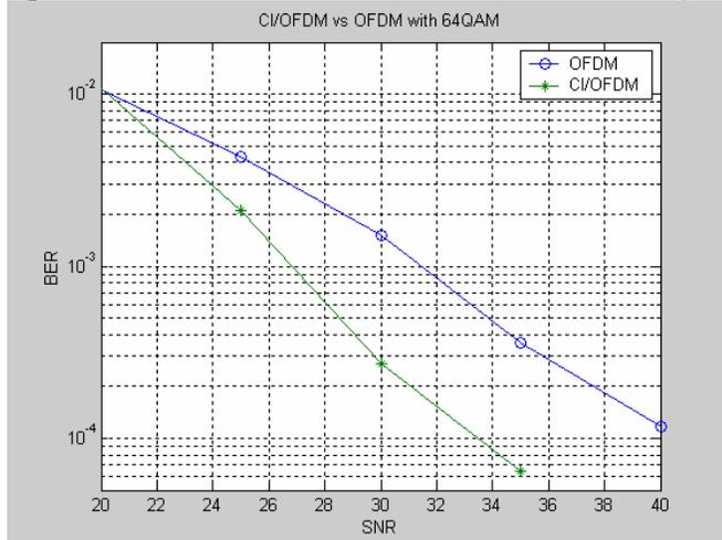
Figure 4. Simulation Results for CI/OFDM with 64QAM
