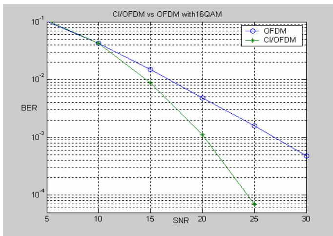
Figure 3. Simulation Results for CI/OFDM with 16QAM
