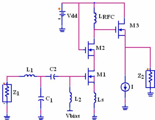
Fig. 4 Overall Schematic of designed LNA
