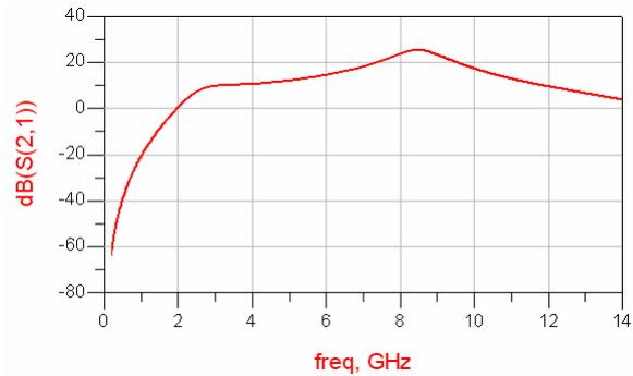
Fig. 6 S<sub>21</sub> or Gain is more than 10dB in Full band of UWB
