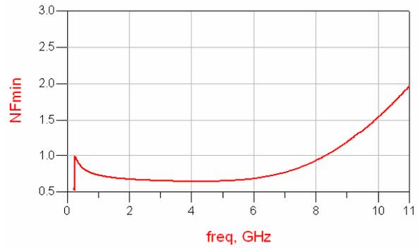
Fig. 5 Noise Figure is less than 1.75dB over the Full band of UWB
