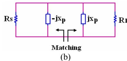
Fig. 2 (a) Illustration of L sub circuits for two stages ladder network. (b) Illustration of matching equivalent for first L sub circuit.
