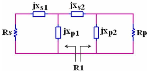
Fig. 1 Two stages LC ladder matching network
